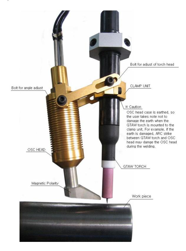
2) How to align the tungsten electrode point and the pole of electric magnetic power.
